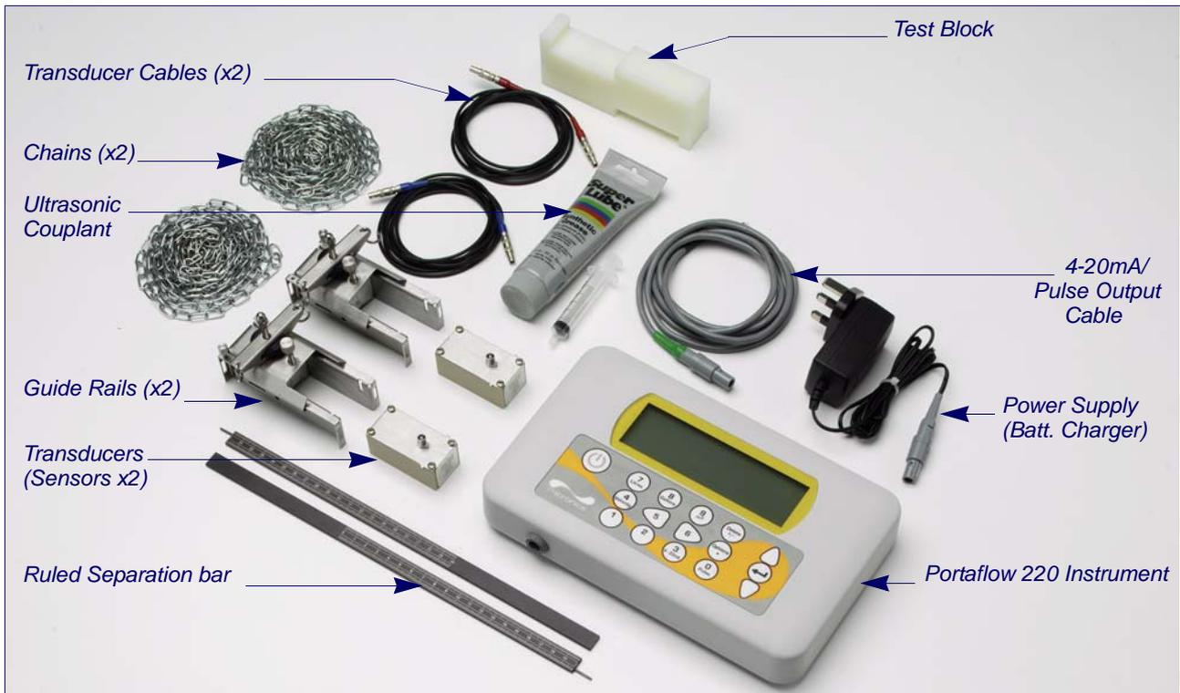
**Figure 1.2 Standard Portaflow equipment**
