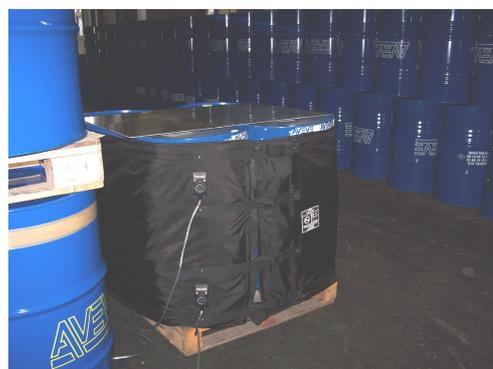
“Prior to the use of the LMK heating jackets, significant delays could be experienced when certain ingredients were used in our manufacturing process. Fitting these cost effective jackets increased our flexibility, reduced down time during product change-over, and helped maintain consistency”
