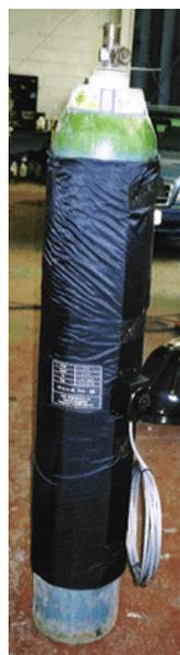
Outer surfaces of each jacket utilize tough, water resistant nylon materials, inner layers are manufactured using unique coated glass cloths for protection from chemicals and long term temperature durability. All heating jackets utilize high efficiency insulation to reduce heat-loss to a minimum, so LMK can also provide unheated insulated covers to fit containers where electrical power is not available.
