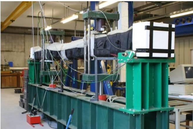
Custom "Hi-Heat" LMK Flexible Heating Jacket on site at Durham
