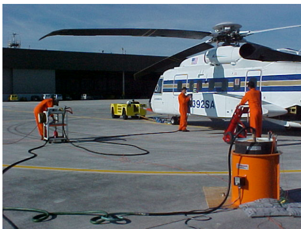
LMK Thermosafe Induction drum heater, with a test Sikorsky S-92 aircraft being fuelled from a barrel of hot JP-8 fuel at 136°F.
