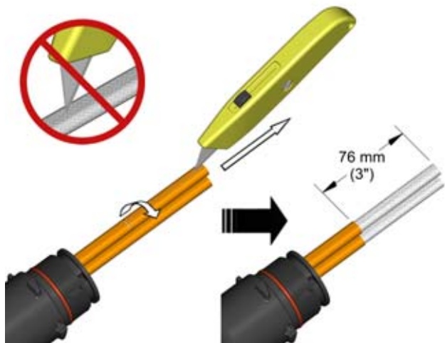
C1. Cut and remove overjacket. Do not cut metallic braid.
